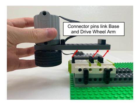
Drive wheel arm in longest configuration. The left image illustrates a large drive wheel fitted to the arm. The right image illustrates a small drive wheel fitted to the arm; this drive wheel will be better served by a shorter arm to minimize its distance to the base.
