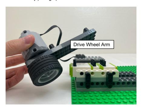
Set length by changing where Base connector pins attach to the Drive Wheel Arm.
