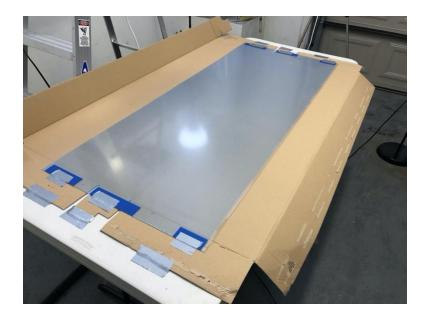
Notice the layering. The acrylic sheet and table are separated by a cardboard sheet to protect the table. The duct tape and acrylic sheet are separated by painters tape to protect the acrylic sheet. Make sure that each layer is firmly in place – shifting during cutting acrylic presents a safety risk.
