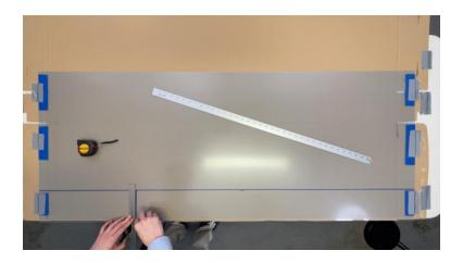
The lengthwise and heightwise lines demarcate the piece forming the sidewall. A metal straight edge is useful for creating straight lines and a tape measure is useful for measuring out the circumference of the lazy susan. Note that the acrylic sheet pictured is much larger than but features the same thickness as the option in the parts list.
