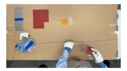
Before sanding the piece forming the sidewall, remove the protective plastic layer and any other coverings – e.g. tape. Use a hand sized patch of 220 grid sandpaper to sand the "rough" or recently cut edges of the sidewall piece until dull.
