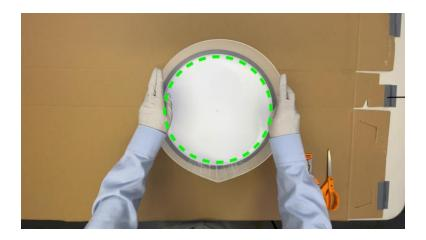
After prior calibration, the homemade acrylic cylinder should fit snugly. Ideally, the teardrop shaped loop will fill the lazy susan such that the prior's outer side is flush with the latter's rim – the ends of the sidewall piece may be slightly inwards. Note that the green ring marks the upcoming bond between the inner side of the homemade acrylic cylinder and floor of the lazy susan.
