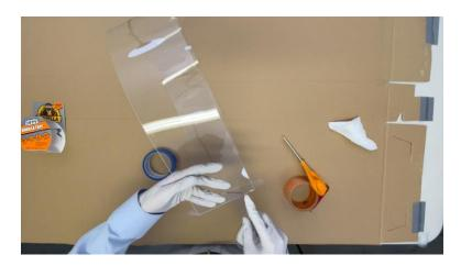
When working with layers of waterproof tape, air pockets below propagate upward. After each application of waterproof tape, use a straight edge (e.g. ruler) to smooth and push out any air pockets in the layer. Some air pockets will be impossible to remove but address as many as possible.
