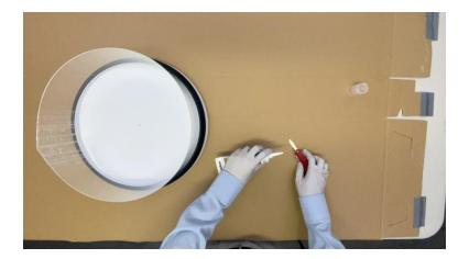
Silicone is packaged in squeeze tubes amongst other containers. Prepare the squeeze tube by cutting off the tip of the applicator.
