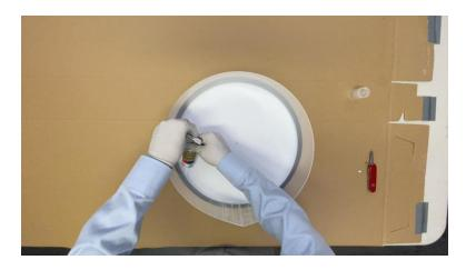
The bond is responsible for preventing the tank's contents, potentially 3.5 gal (13.25 L) of liquid, from leaking through the bottom. Thus, be generous when applying silicone to ensure that the entire contact is covered – the DIY Sidewall Tank prototype features a pencil diameter stream of sealant.
