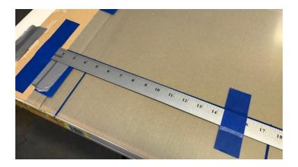
Starting from an end, align the metal straight edge to an edge of the line. This ensures that the cut remains parallel, rather than at an angle, to the "clean" edge. Use painters tape to fix the metal straight edge in place.
