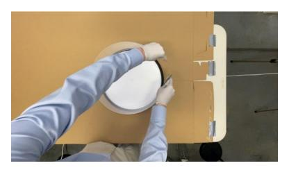
The sidewall piece is thin enough to bend into the shape of the lazy susan. We bend then place the sidewall piece into the lazy susan to gauge its fit before connections are made. The sidewall piece is fixed within the lazy susan because the latter features a raised rim. Nevertheless, until its ends are connected with waterproof tape, do not allow the sidewall piece to rest inside the lazy susan without support.
