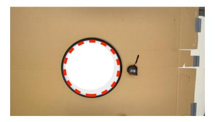
Silicone will be applied twice to form redundant seals – outer and inner. Here, we bond the rim of the lazy susan to the outer side of the homemade acrylic cylinder. Follow the edge between the rim and floor of the lazy susan – marked in red. Later, we bond the inner side of the homemade acrylic cylinder to the floor of the lazy susan. Note that the prototype DIY Sidewall Tank omits the prior silicone application.
