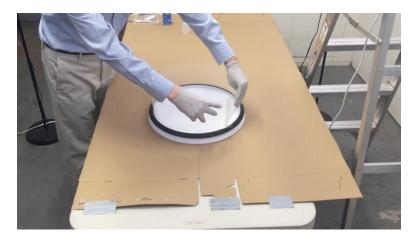
Once the loop is completed within the lazy susan, check for any overlap between sidewall piece ends. The ideal situation is for sidewall piece ends to continue along the same curve rather than overlapping (too long) or forming a teardrop shape (too short).
