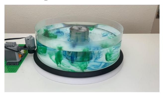
The DIY Sidewall Tank provides an affordable yet effective large cylindrical tank for the DIYnamics LEGO-Based Tables. The DIY Sidewall Tank presents an alternative to the Sidewall Tank. Both approaches affix an acrylic cylinder onto a lazy susan to create an integrated rotating tank platform. The tanks offer greater diameter and height than the default option thus expanding the experimental possibilities of the model.
