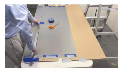
Scoring consists of dragging the plastic cutter along the metal straight edge and applying pressure to carve material from the acrylic sheet. In the direction comfortable for you, pull the blade back repetitively. Note that your hand should always be ahead or out of the potential path of the blade.
