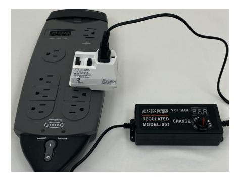
Step 5: Rotate the Adjustable Power Supply Adapter's dial to adjust the voltage provided to the LEGO Assembly's motor. The motor is rated for 9V; proceed above 9V at your own risk.
