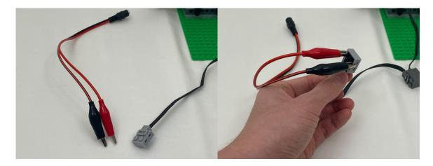
Ensure that the alligator clips contact the light gray end's metallic strips on its interior.
