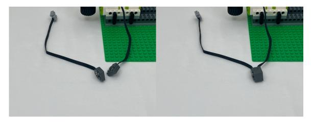
Step 2: Attach the Power Jack to Alligator Clip Connector's alligator clips to the Extension Wire's light gray end (highlighted in green).
