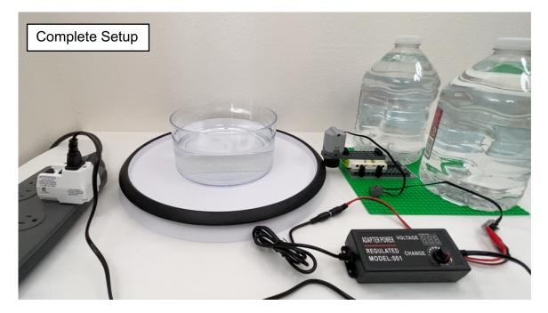
Step 1: Connect the LEGO Assembly's wire to the Extension Wire's dark grey end (highlighted in red).
