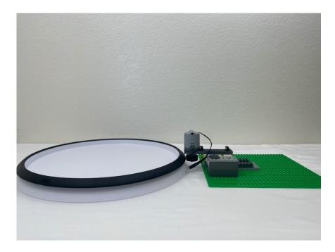
Ensure that only the drive wheel is in contact with the turntable's black rim. A lack of or unwanted contact can inhibit the drive wheel from smoothly rotating the turntable.
