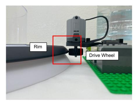
Ensure that the drive wheel arm is directed towards the turntable's center.
