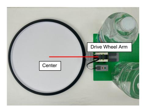
Step 3: Place Weights on the baseplate to hold the LEGO Assembly firmly in place in contact with the OXO Lazy Susan. We use water bottles as Weights but other heavy items are suitable as well.
